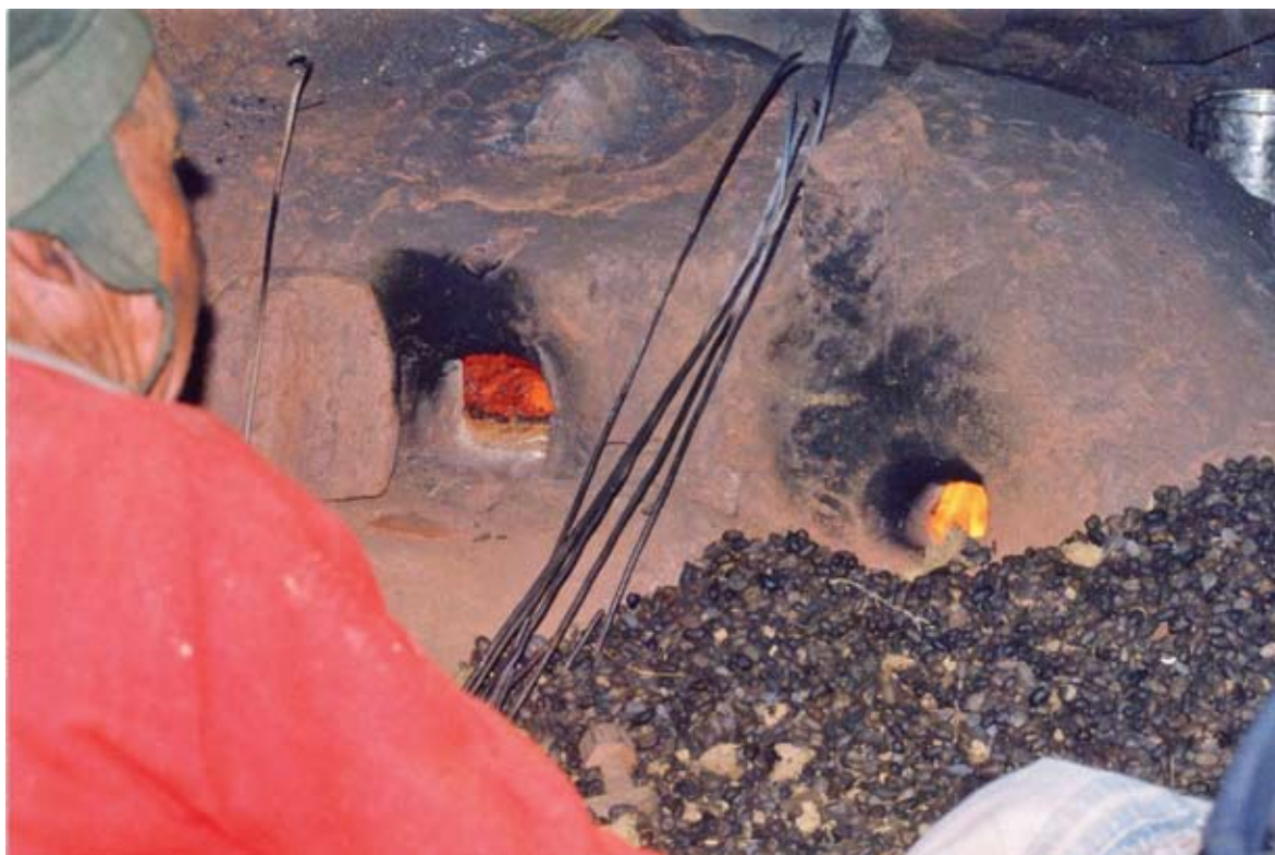
Figure 5. Modern cupellation hearth used by Carlos Cuiza to refine silver. The opening to the fire box can be seen to the right; the door to the hearth itself is on the left.
