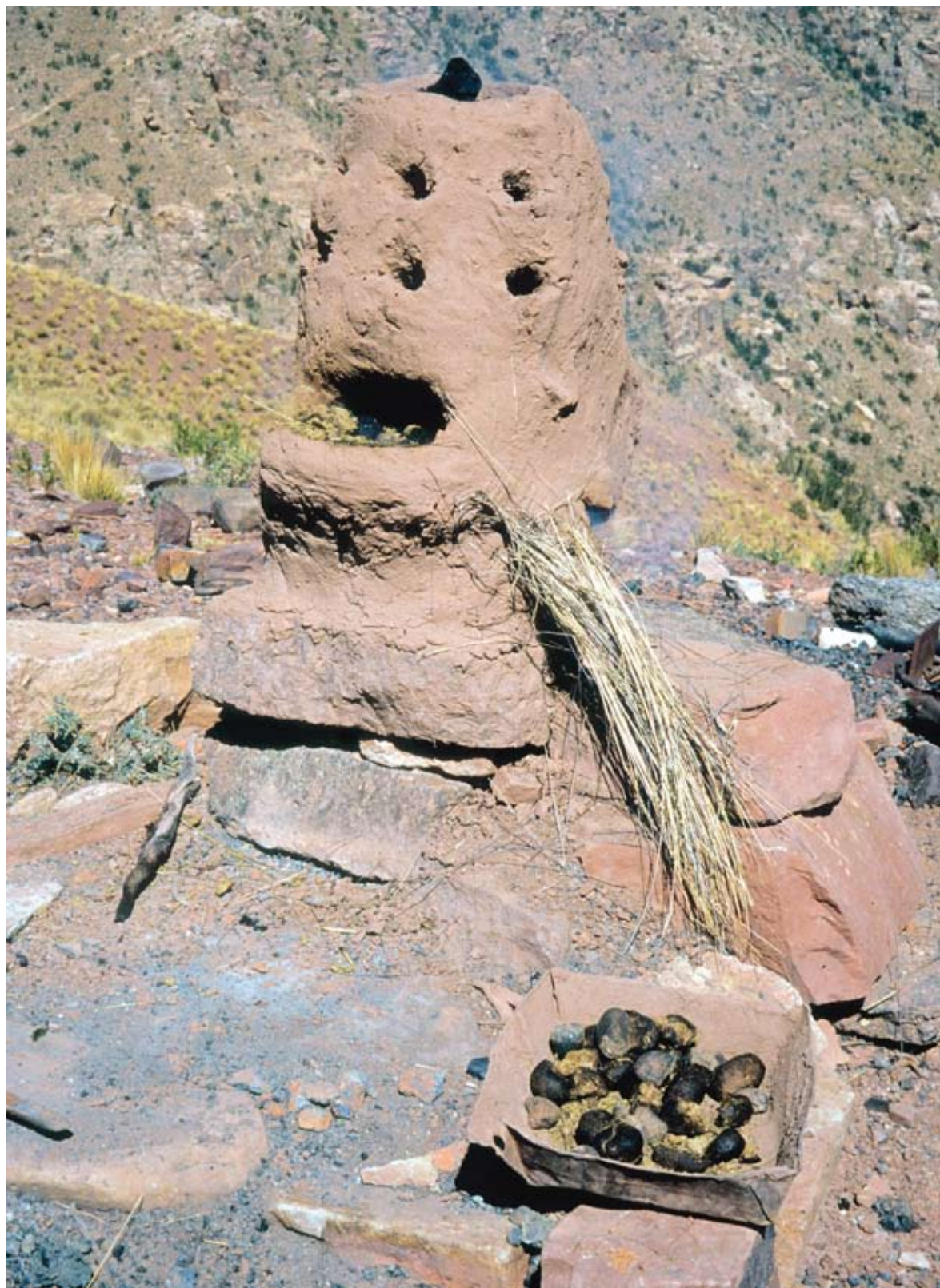
Figure 4. Modern huayrachina used by Carlos Cuiza to produce lead metal.
