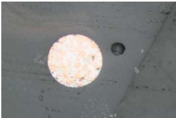
Figure 9. Sample TR4000-L3-SL01: prill with copper and lead intergrown (photo by C. Zori).
